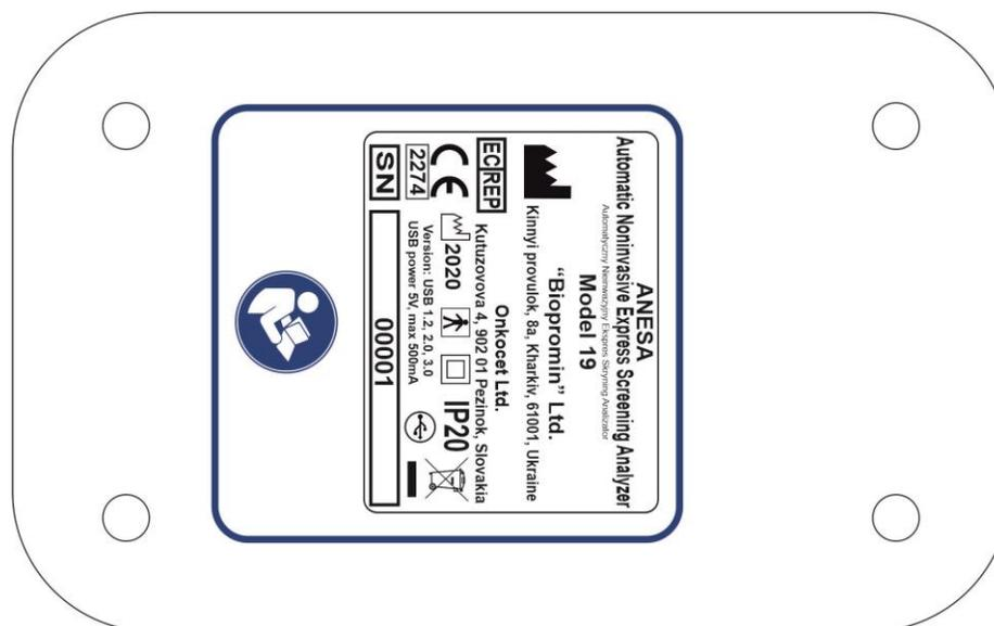
Project of the **main label** for the MD ANALYZER (sample is made with the label for the MD with name ANESA)\*
